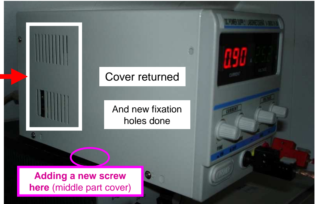
Modified cooling near back-side + greater hole near radiator output
