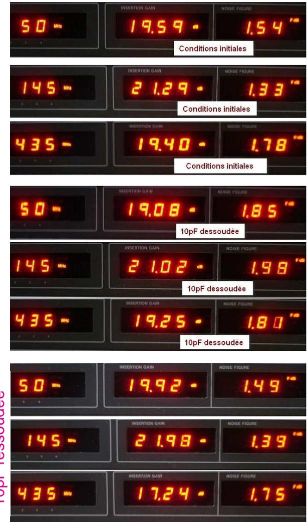
It can be also used with an UHF IF but its gain/Nf performance is more optimised at 144 MHz
