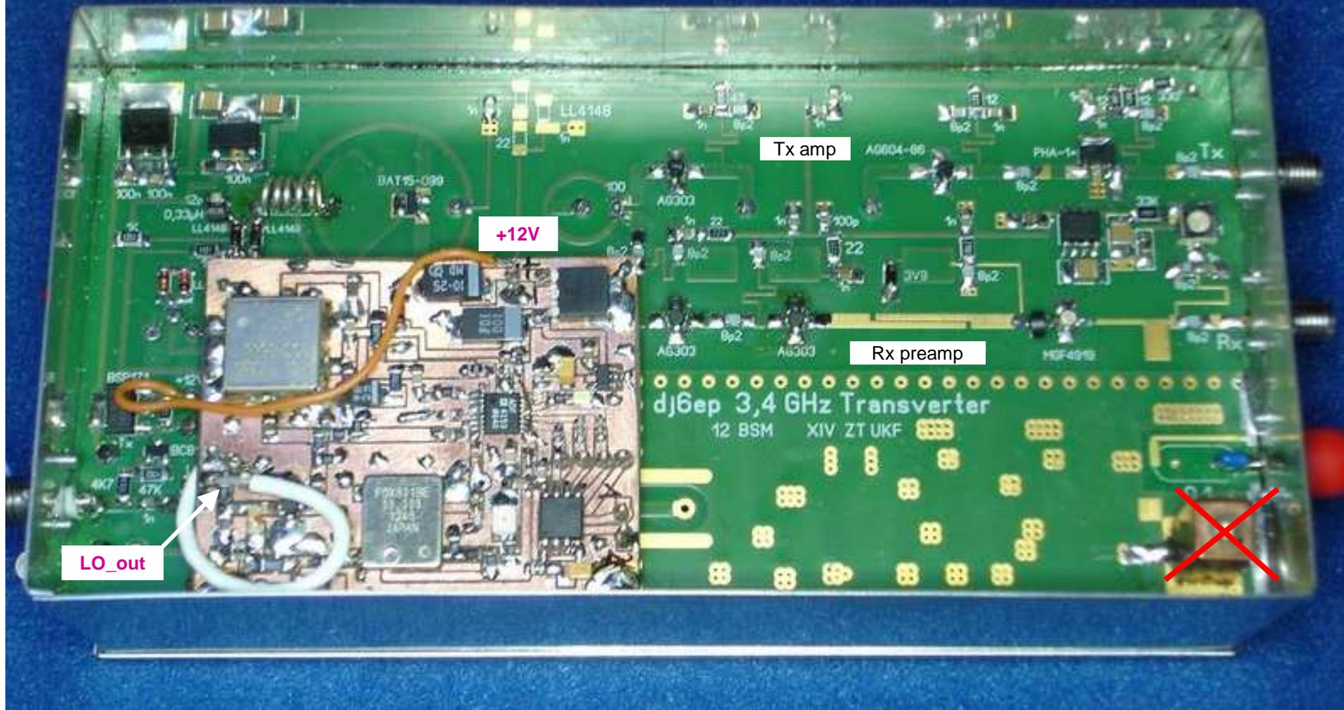
The DF9NP LO output is soldered after the strap desoldering (page 27)
