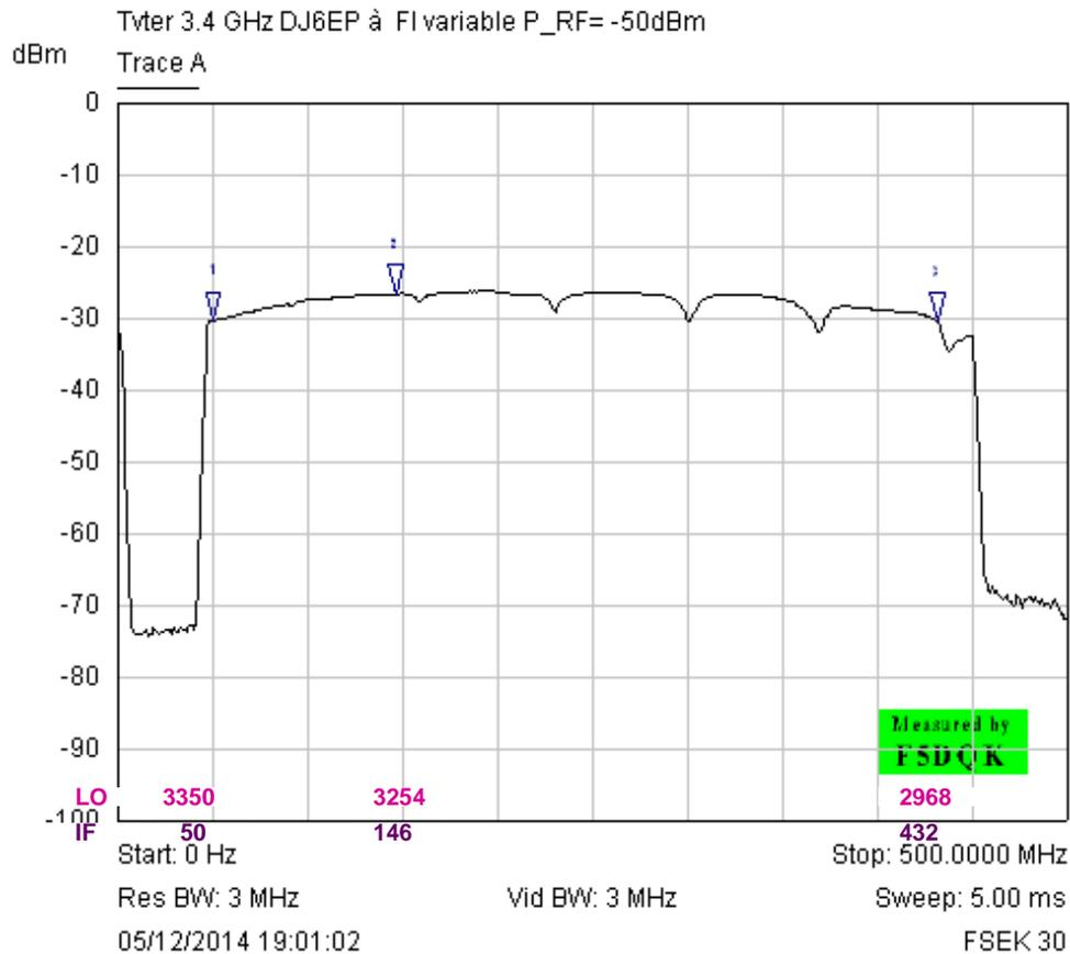
With RF=3.4 GHz, this is the IF conversion gain as function of LO variable frequency (with initial IF diode switching)
