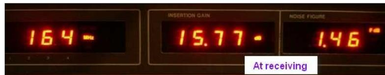
*B/ TRx common bell filter adjusting (vy hard to do)*
