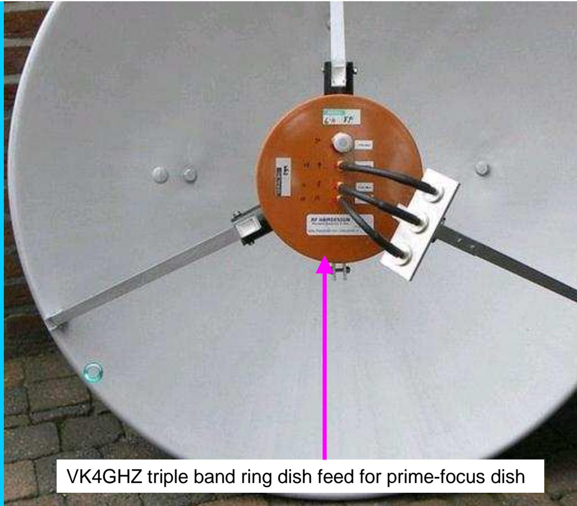
VK4GHZ triple band ring dish feed for prime-focus dish
