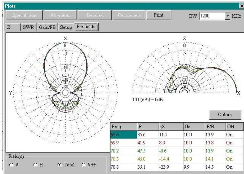
Gain shown here is in dBi (utopic and not exploitable). That's the dBd value + 2.15 dB
