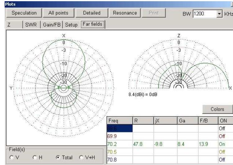
SWR and F/B ratio at both frequencies
