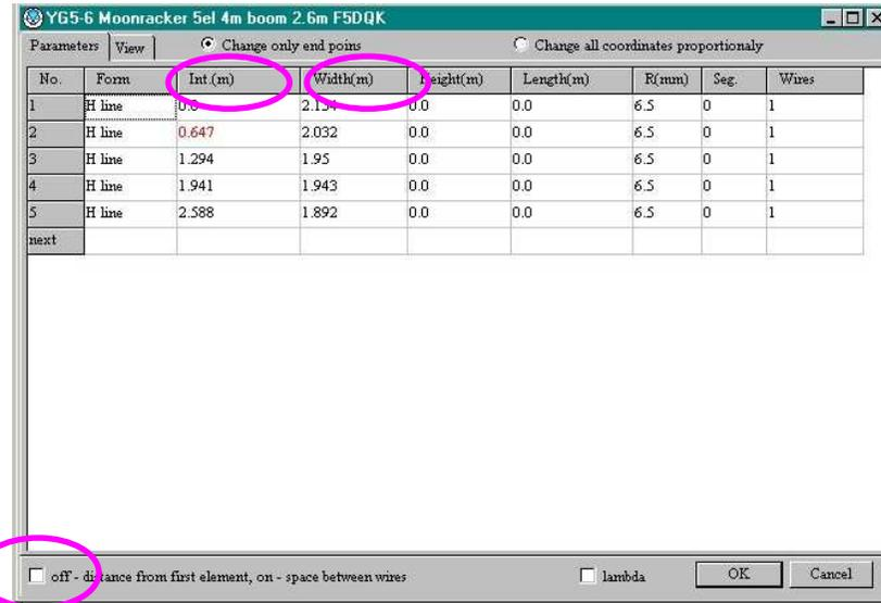
Gamma, té match, hairpin have to be hand drawn. In this case, you must also enter an equivalent serial capacitor. SWR 'll be affined by entering more times new values of C in pF, and adjusting the gamma diameter and spacement to the dipole
