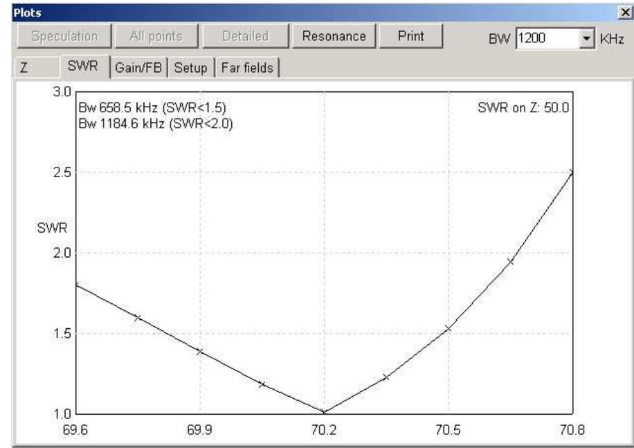
You can also try to lengthen or straighten the boomlength in order to see its influence on gain while keeping at 50 Ohms impedance, but the **best gain compromise is only obtained with 3.60 M total boomlength !!!**
